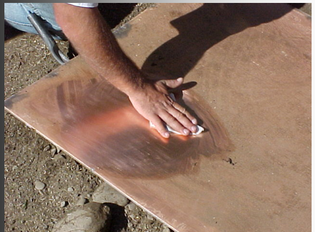
As-bonded Copper-Stainless Plate
